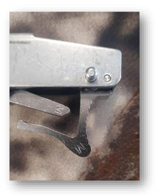
Trigger mechanisms with the "M" have already been updated at the factory - **No further action required**
